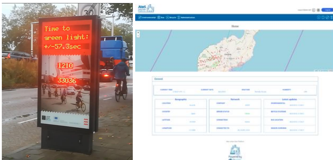
Figure 27 Eindhoven's finished product: Road-Side display, showing the time to green use case for passing cyclists; AUDP – Home and Map Dashboard
