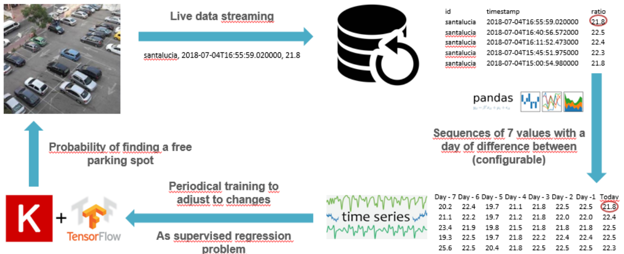
Figure 4: Data flow over AI Prediction Engine, example configuration
